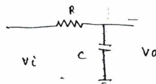
$$\frac{V_o(s)}{R(s)} = \frac{V_o}{V_i} = \frac{1}{C(1+Rs)} = \frac{1}{1+Ts}$$
