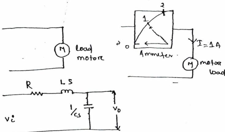
$$\frac{V_o}{V_i} = T(s) = \frac{\frac{1}{Cs}}{R + LS + \frac{1}{Cs}}$$
